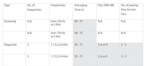
3 configurable protocols Frequency bands: 0.7 to 5 kHz Stimulus intensity: 70 - 90 dB pe SPL Customizable fields are indicated in GREY: For any additional information please contact: support@resonance-audiology.com
